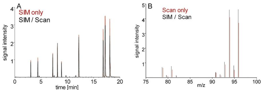
**Fig. 5.** (A) Comparison of SIM chromatograms of 9 compounds (bromomethane, dichloromethane, 1,2-dichloroethane, tetrachloromethane, 1,2-dichloropropane, toluene, ethyl benzene, *m*- and *p*-xylene). (B) Mass spectra of bromomethane in Scan mode and combined SIM/Scan mode.
