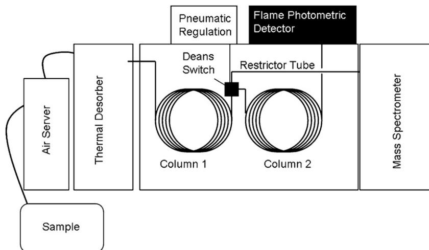
Fig. 1. Scheme of the TD-2D-GC-MS/FPD system.
