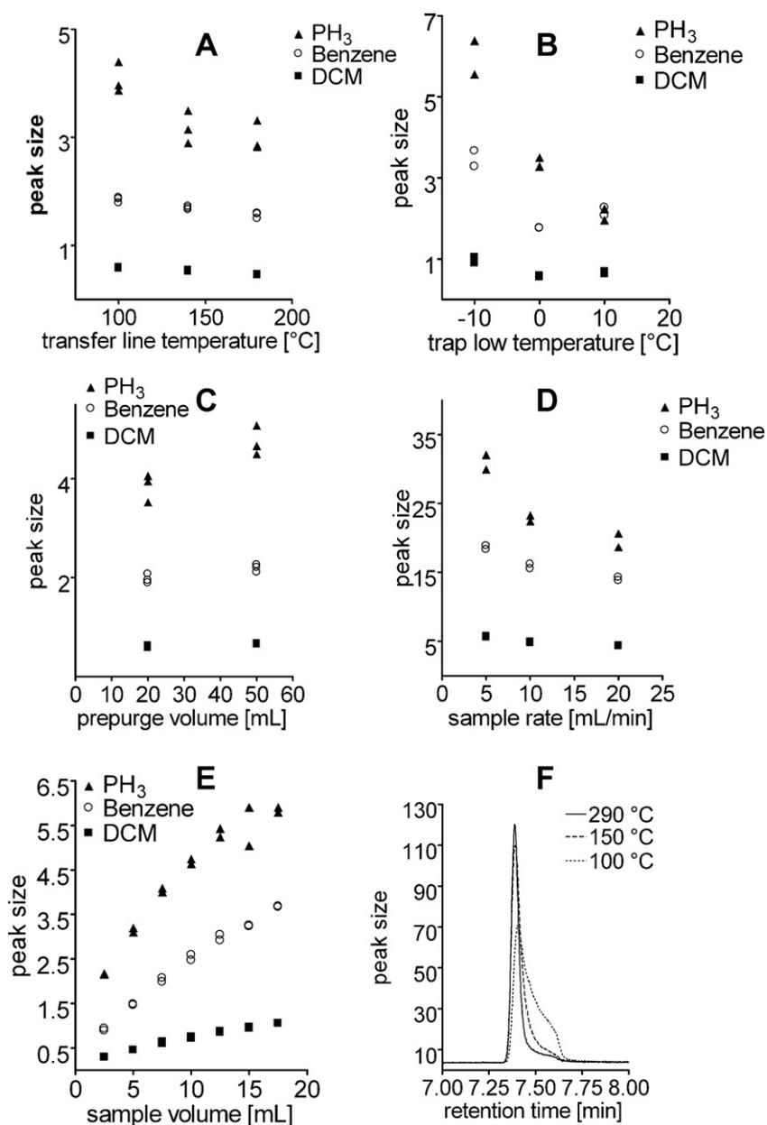
**Fig. 2.** Influence of different thermal desorption parameters on peak size for phosphine (PH<sub>3</sub>, 150 μL m<sup>-3</sup>), benzene (100 μL m<sup>-3</sup>) and dichloromethane (DCM, 100 μL m<sup>-3</sup>) (A–E). Influence of trap heating temperature on the peak shape for phosphine (F); note the different scales for the peak size.
