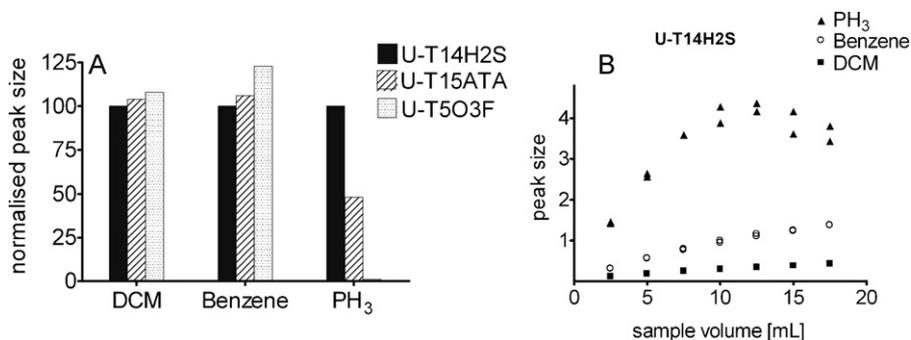
**Fig. 3.** (A) Comparison of three different cold traps for benzene ( $100 \mu\text{L m}^{-3}$ ), dichloromethane (DCM,  $100 \mu\text{L m}^{-3}$ ) and phosphine (PH<sub>3</sub>,  $150 \mu\text{L m}^{-3}$ ); (B) Determination of breakthrough volume for the U-T14H2S cold trap.
